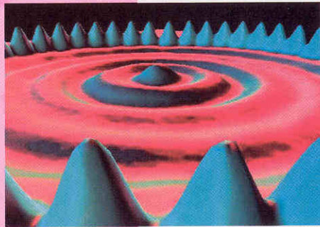
subatomic sculpture By making a ring of atoms to act as a "corral," researchers in the 1990s were able to trap electrons as waves moving across the surface of a metal like ripples on the surface of a pond.
