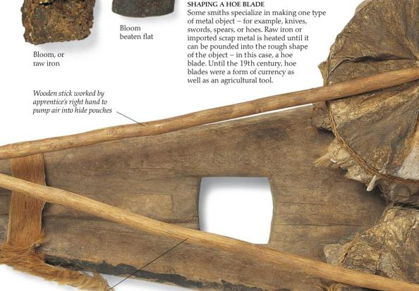
left hand -TOOLS OF THE TRADE The smith's equipment consists of hammers, chisels, an anvil, and bellows. Air is pumped through the bellows by the smith's apprentice or a young male member of the family. This air controls the fire, and therefore the temperature at which the metal is heated. The hot metal is beaten into shape on the anvil with a hammer. The smith frequently returns the metal to the fire until the task is completed. Although the tools used are
