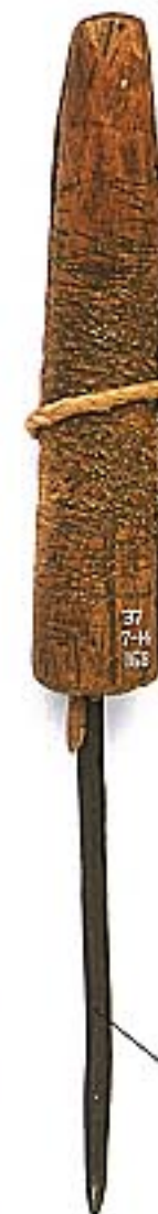
DRILL Carpenters often used a bow drill to make holes for pegs to join pieces of timber together. The wooden shaft of this bow-drill is well worn - it was obviously much used by its original owner.
