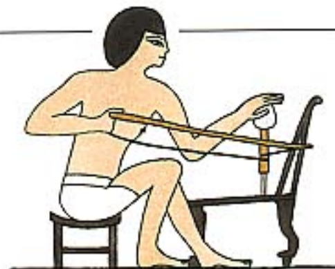
BORING JOB To bore a hole in a plank of wood the carpenter used a drill consisting of a metal or flint point in a shaft of wood. He placed it over the spot in the plank where he wanted the hole and rotated the cutting point using a bow. Sometimes a workmate would hold a heavy pebble over the shaft of the drill to create more pressure.
