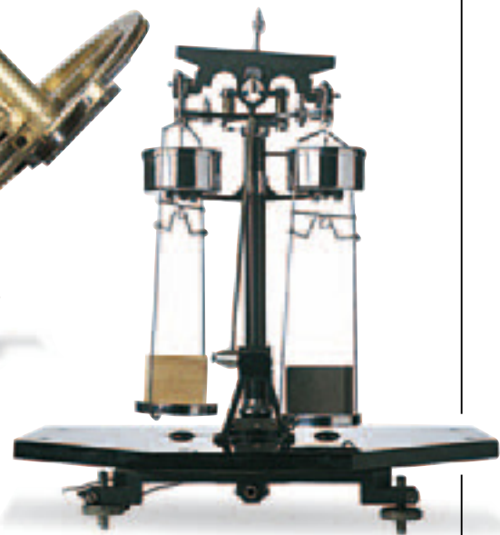
Beam balance to find mass
