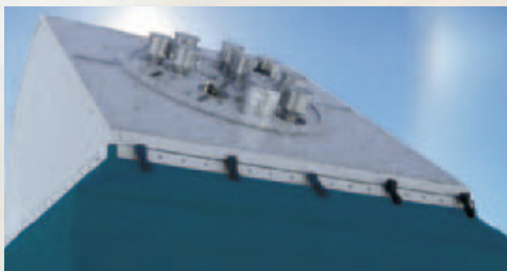
Solar array shields telescope from Sun's heat
