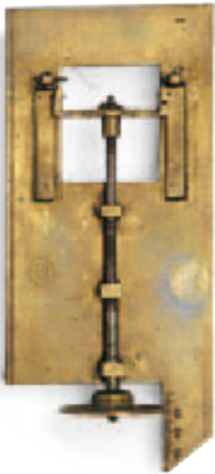
Micrometer for use with a telescope
