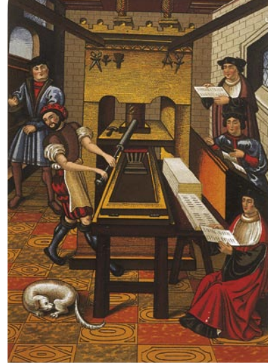
IN THE WORKSHOP The bustle of a printing office was very different from the quiet of a medieval scribe's desk. This 16th-century picture shows everyone hard at work. The compositor sets type, the printers operate the press, and the proofreader checks a printed page for errors. Only the dog is asleep.
