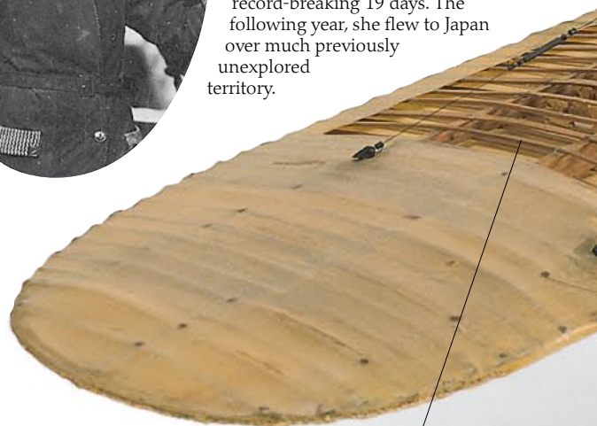
Wooden spars to shape and strengthen wing
