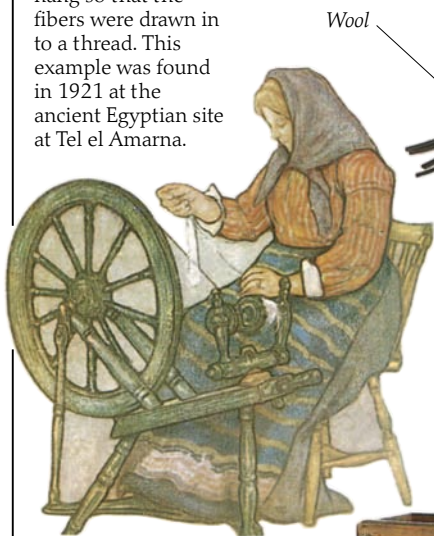
SPINNING AT HOME The spinning wheel, which was introduced to Europe from India about A.D. 1200, speeded up the spinning process. In the 16th century, a foot treadle was added, freeing the spinner's hands – the left to draw out the fiber, the right to twist the thread.
