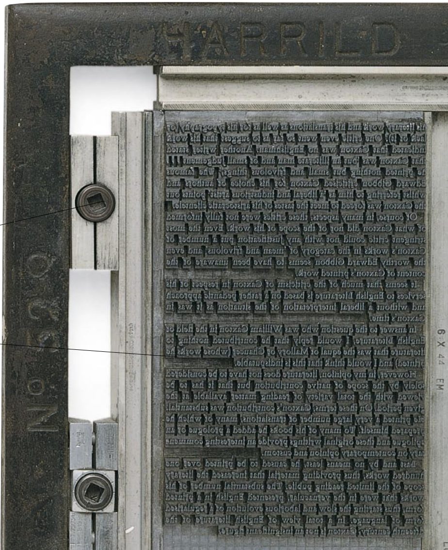
Adjustable grip to set width of lines
