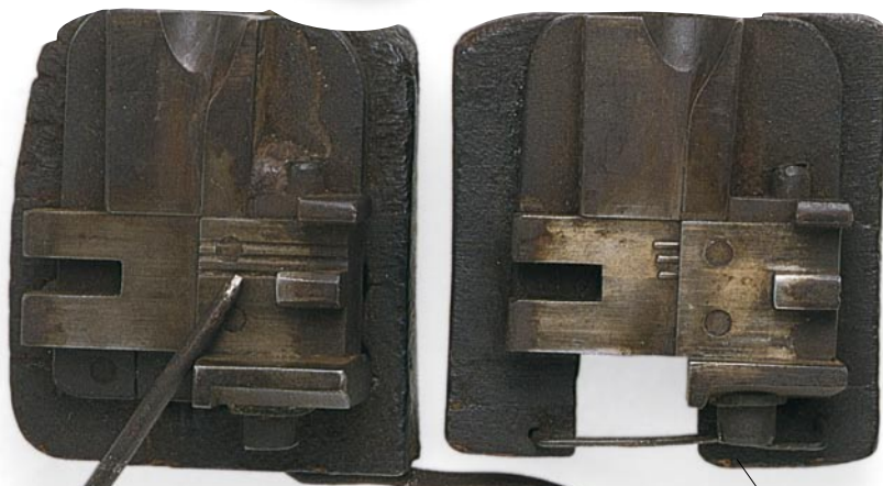
TYPE MOLD The matrix was placed in the bottom of a mold like this. The mold was then closed, and the molten metal was poured in through the top. The sides were opened to release the type.
