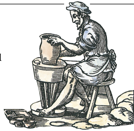
POTTER'S WHEEL By 300 B.C. the Greeks and Egyptians had invented the kick wheel. The disk's heavy weight meant that it turned at near constant speed.
