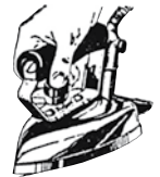
ELECTRIC IRON The first electric iron was heated by an electric arc between carbon rods and was highly dangerous. A safer iron was patented in 1882. It used an electrically heated wire element like the coils on a stove.
