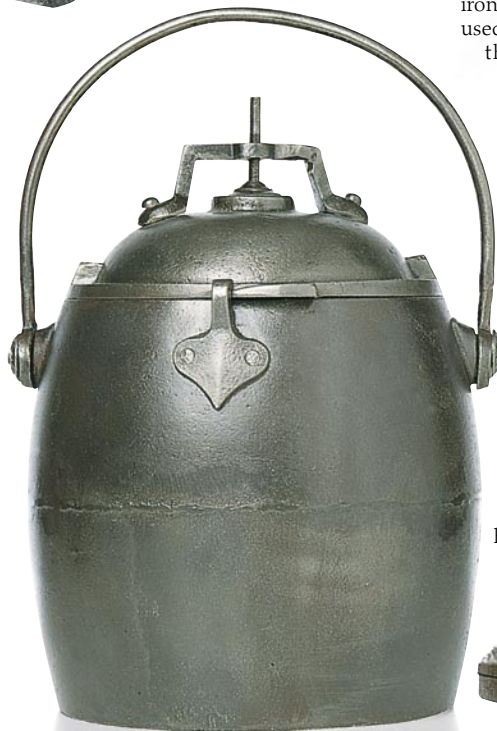
QUICK COOKING left The pressure cooker was invented by Frenchman Denis Papin in 1679. He called it the "new digester." Superheated steam at high pressure formed inside the strong container. The high temperature cooked the food in a very short time.
