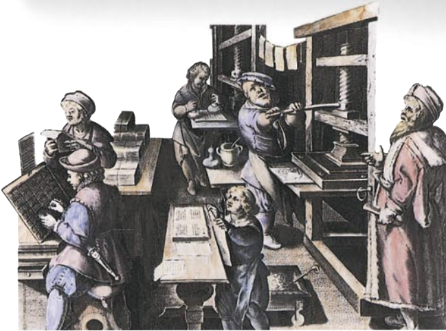
Screw locks type in place
