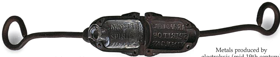
Open and shut mold for making apothecaries' vials (19th century)
