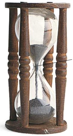
SANDS OF TIME The sandglass was a simple timing device, which allowed scientists to work out how fast objects fell, or how long it took for chemicals to react. More accurate measurements of time were not possible until after the first pendulum clock was made in 1657.
