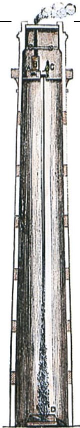
DROPPING LEAD Bullets and lead shot used to be made by letting drops of molten lead fall from the top of a "shot tower." While still liquid, the lead droplets formed spheres, and then "froze" in this shape.
