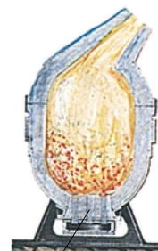
Air blown through inlets and carbon burned off
