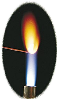
FLAME TEST Here common salt (sodium chloride) burns yellow in a flame, revealing the presence of the element sodium.
