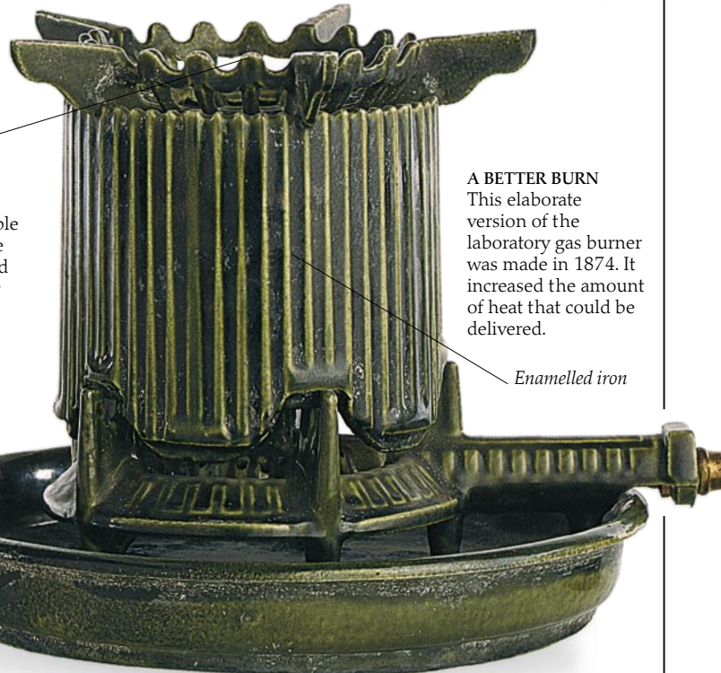
Air is forced through the thin metal tube
