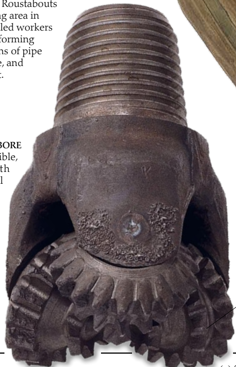
Wheels of drill bit bite into rock as they rotate
