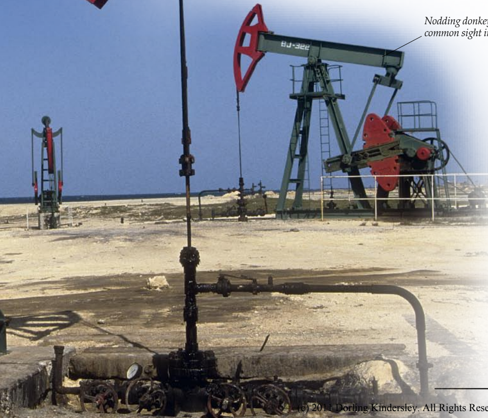
Driving beam operates the plunger in the well shaft as it rises and falls
