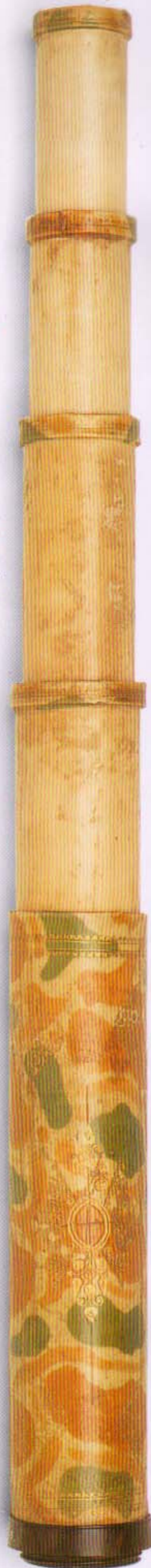
Late-17th-century telescope with tube of paper and vellum
