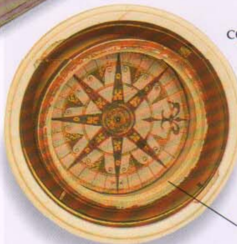
Compass bowl swung in pivoting rings, or gimbals, to keep it level at sea
