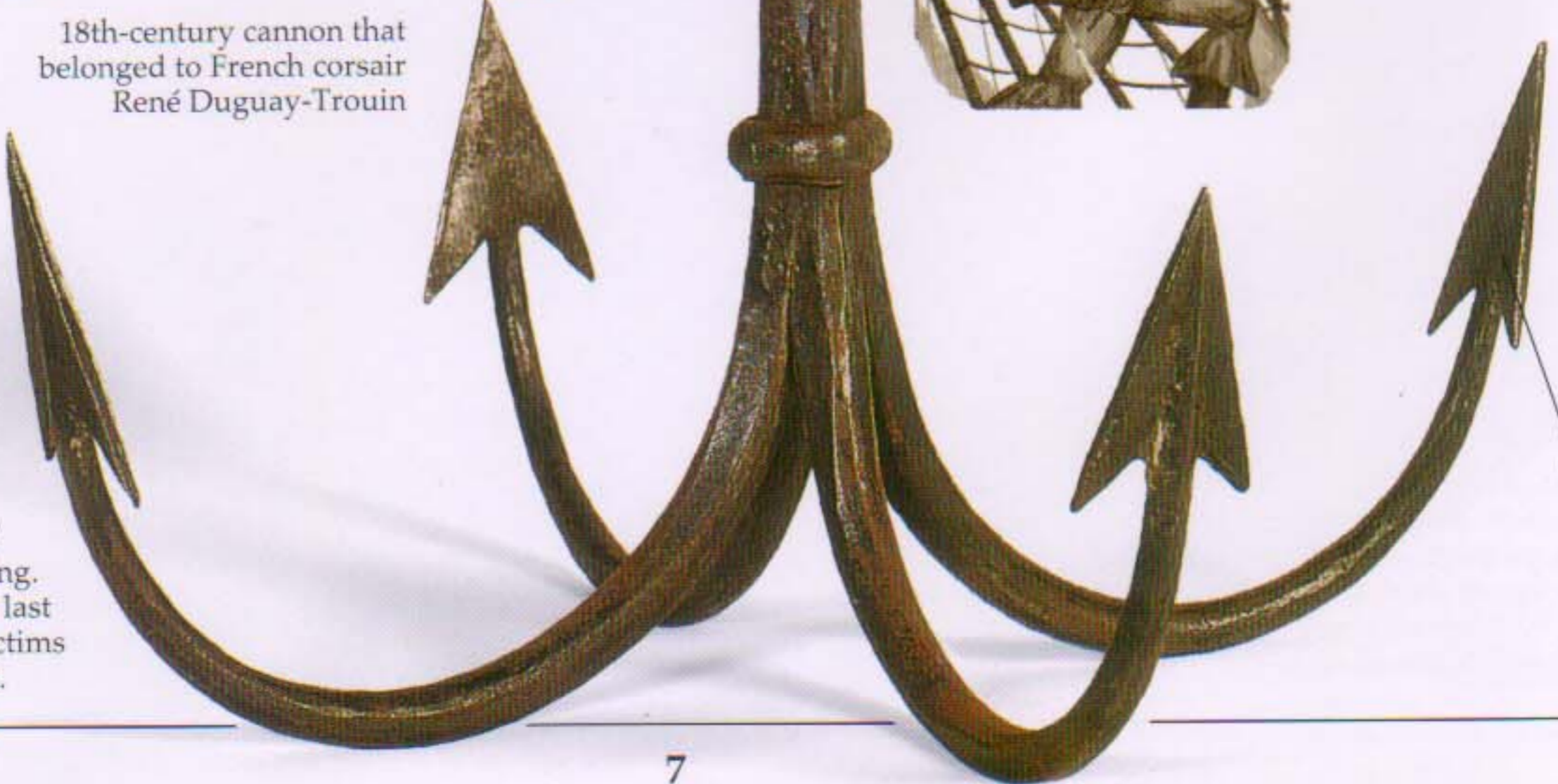
Barbed points are designed to lodge securely in the rigging of another ship
