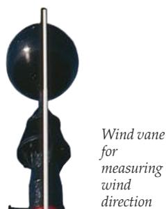
Wind vane for measuring wind direction
