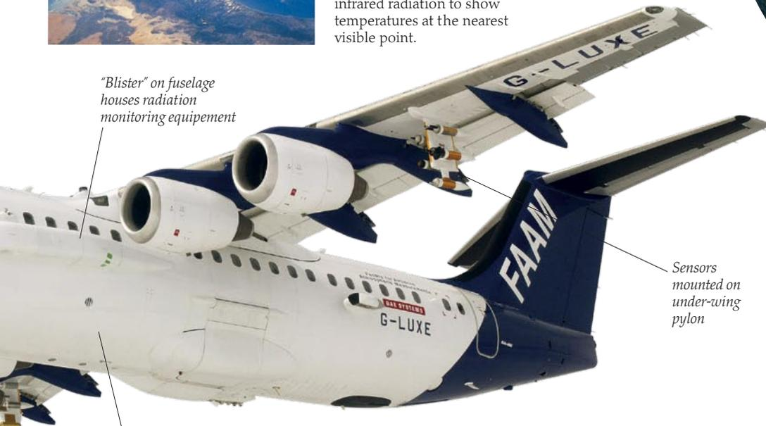
"Blister" on fuselage houses radiation monitoring equipment
