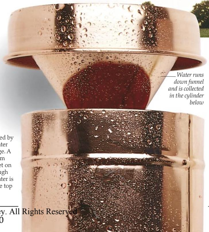
*Water runs down funnel and is collected in the cylinder below*
