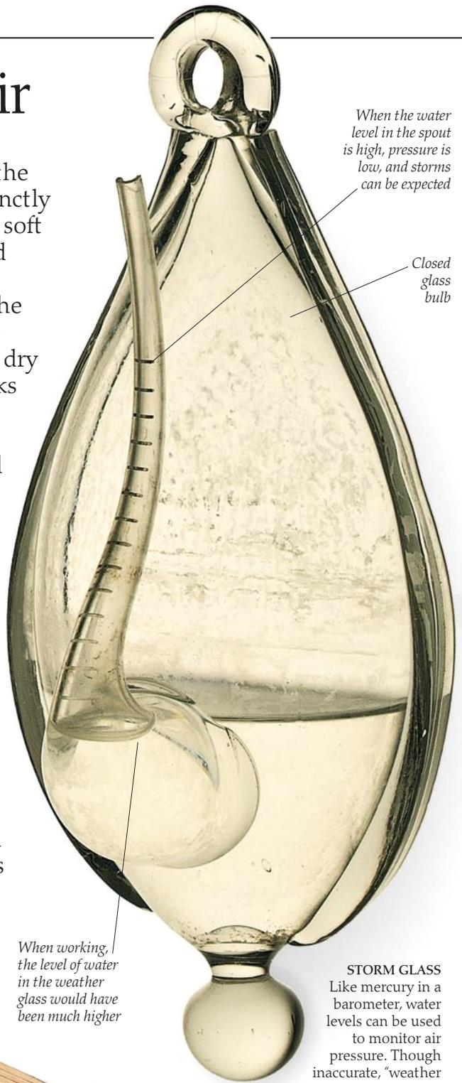
When the water level in the spout is high, pressure is low, and storms can be expected
