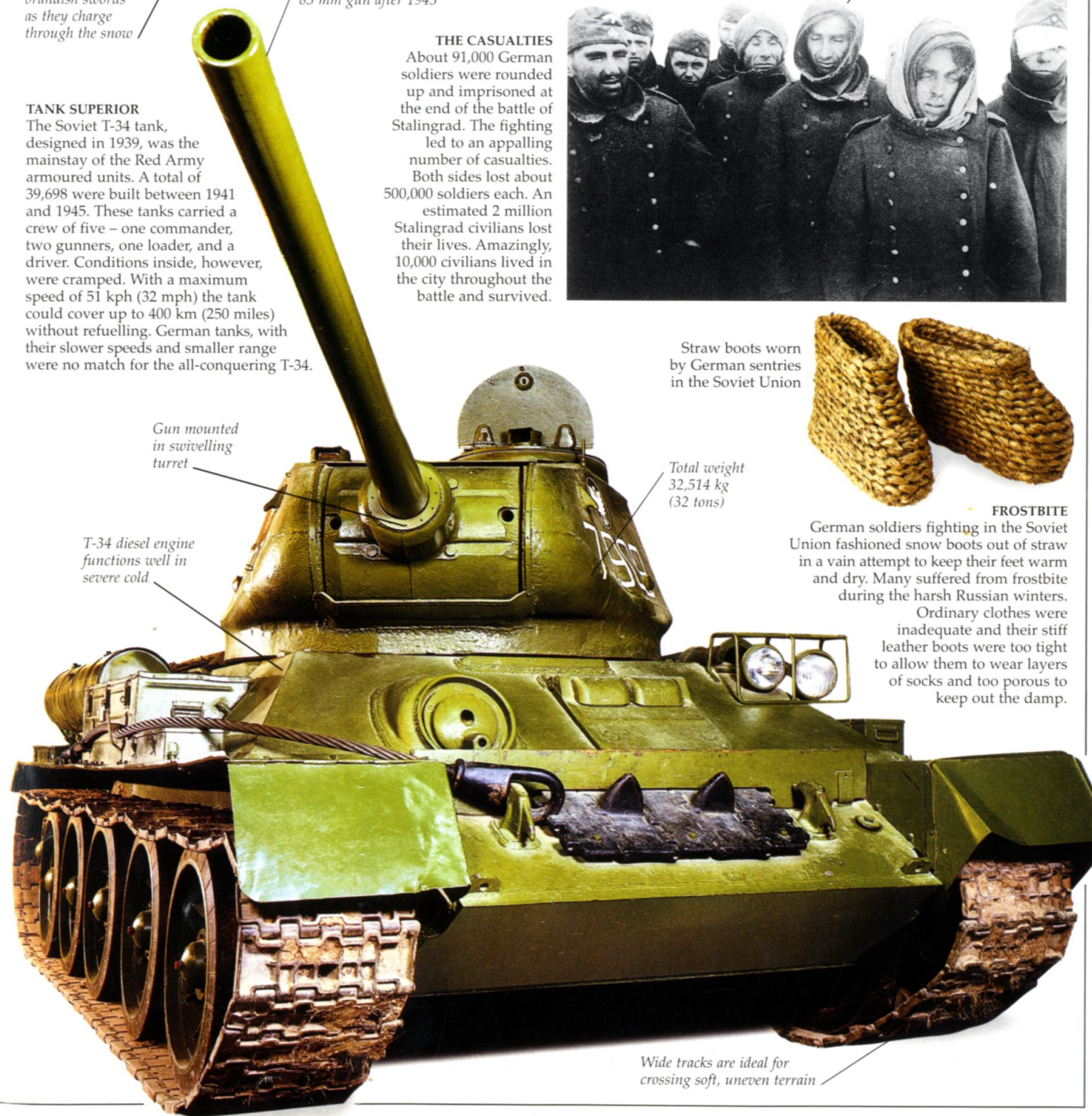
T-34 was armed with an 85 mm gun after 1943
