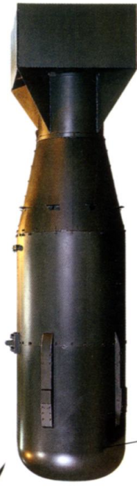
Little Boy was 3 m (10 ft) long with a diameter of 71 cm (28 in)
