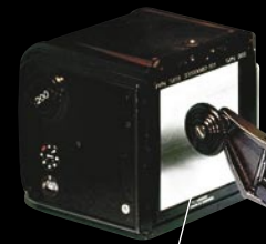
Detachable film magazine – the part that came back to earth
