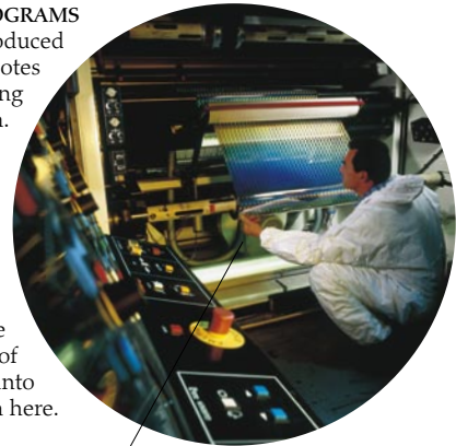
Checking quality of embossed holographic foil
