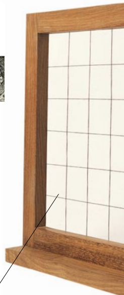
DRAWING THE NET To help him create perspective in his drawings, Alberti devised a “net.” The idea was developed by the German artist Albrecht Dürer in 1525. The net was a square network of black threads stretched on a wooden frame. The artist placed an eyepiece at a fixed distance from the object he was drawing. He then looked over the eyepiece and through the net, and reproduced the outlines of the model onto a sheet of paper with squares corresponding to the network on the frame.
