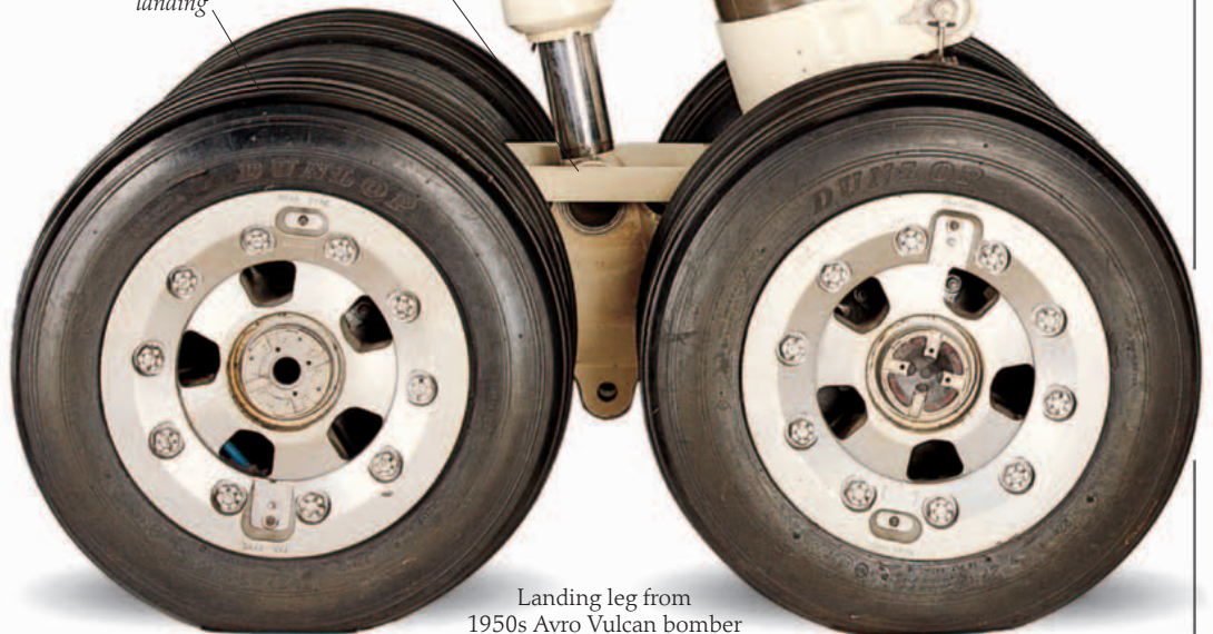
Tires designed to stand enormous loads and huge heat buildup on landing
