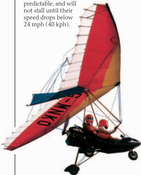
Plastic trike cockpit outer shell on aluminum-alloy tube frame
