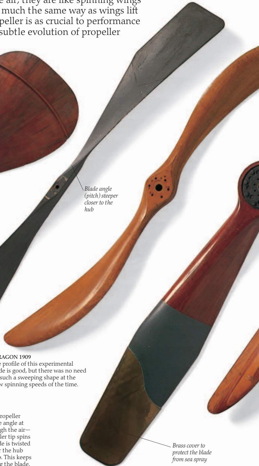
Propeller blade made from strips of wood
