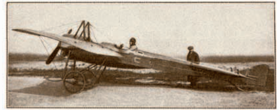
DEPERDUSSIN 1909 The French Deperdussin company was one of the most advanced aircraft manufacturers in the years before World War I, and its sleek monoplanes took many speed records. Despite this, the example above shows many features typical of the pioneering planes, with lateral control by wing-warping, (p. 14), a low-powered engine, and extensive wire bracing.
