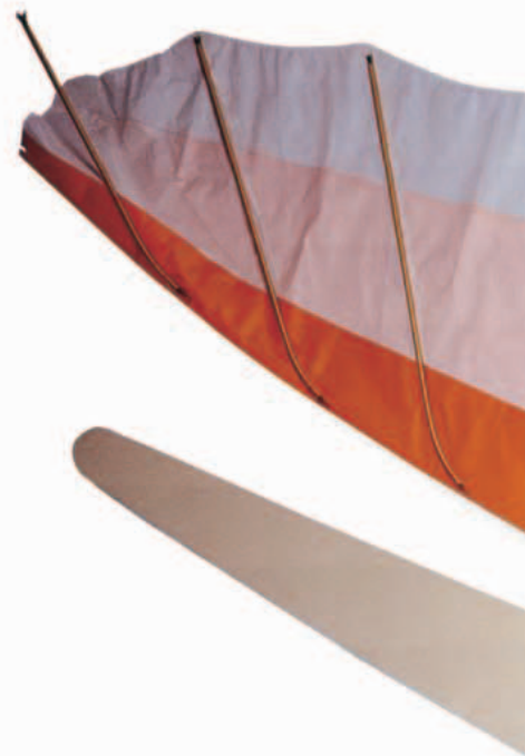
WIDE WING Like the hang-glider on pages 60–61, a flex-wing ultralight like this Solar Wings Pegasus Q has a shallow triangular wing made of Dacron. But it is broader than the hang-glider in order to lift the extra weight of the engine, trike, and two crew members.
