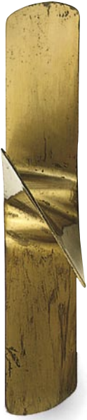
BLADE EDGES The blades of a propeller (in this case a common screw) are helices – like sections of a spiral.
