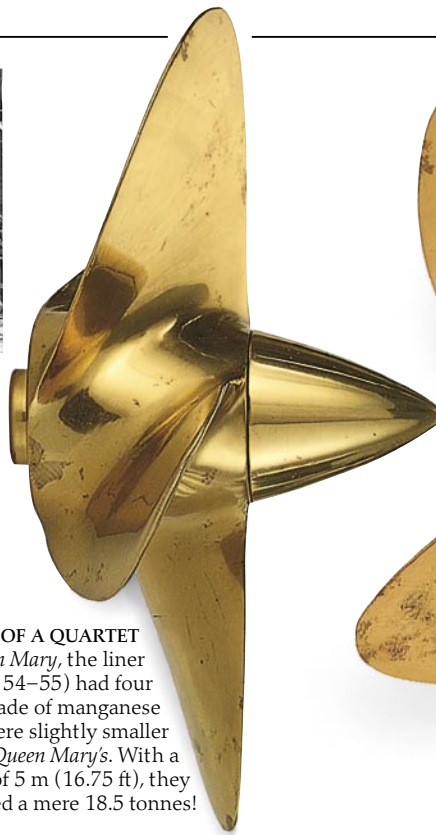
FIT FOR A QUEEN Each of the Queen Mary's (p. 55) four propellers was 5.5 m (18 ft) in diameter and weighed 35 tonnes. Cast in London, the monster screws were then shipped to a yard on the River Clyde for fitting.
