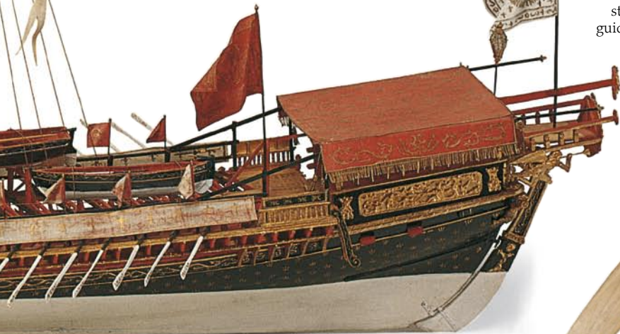
FRENCH STYLE Built in the late 17th century, this French galley was propelled by 60 oars and two lateen sails (p. 25). Galleys were popular with Algerian pirates, and the French copied some of their craft. Like the Greek galley, this one has a ram. A few galleys were merchant vessels, but most were warships. The last battle between galleys was fought at Lepanto in the eastern Mediterranean in 1571. But because they were very fast over short distances, the French navy still had war galleys at the beginning of the 19th century.
