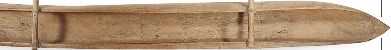
Boom lashed to hull through holes drilled in logboat
