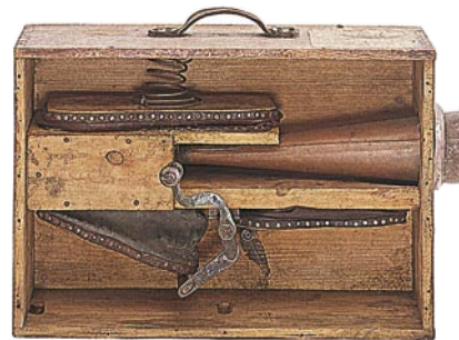
This fog horn uses a cylinder of compressed air to make an ear-piercing noise. As well as warning of a ship's presence, it can be used to signal simple messages. Flares are distress signals and help to guide searching rescue craft.
