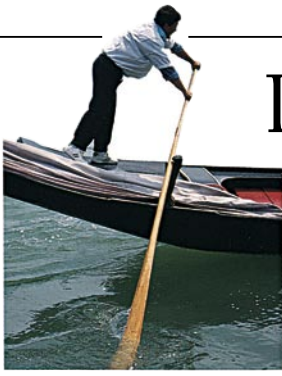
CROOKED CONSTRUCTION The gondola is fatter and wider on one side, the port side, than the other. This means the gondolier can row with one oar and still go in a straight line.
