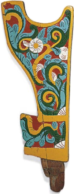
BOOM CRUTCH This practical device comes from an Indonesian jukung from Madura. Its central notch supports the boom whenever the sail is lowered.
