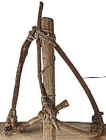
Wooden "double U" connectives that join boom to float
