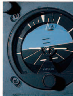
With the sighting string dipping right below the horizon, the plane is rolling right.
