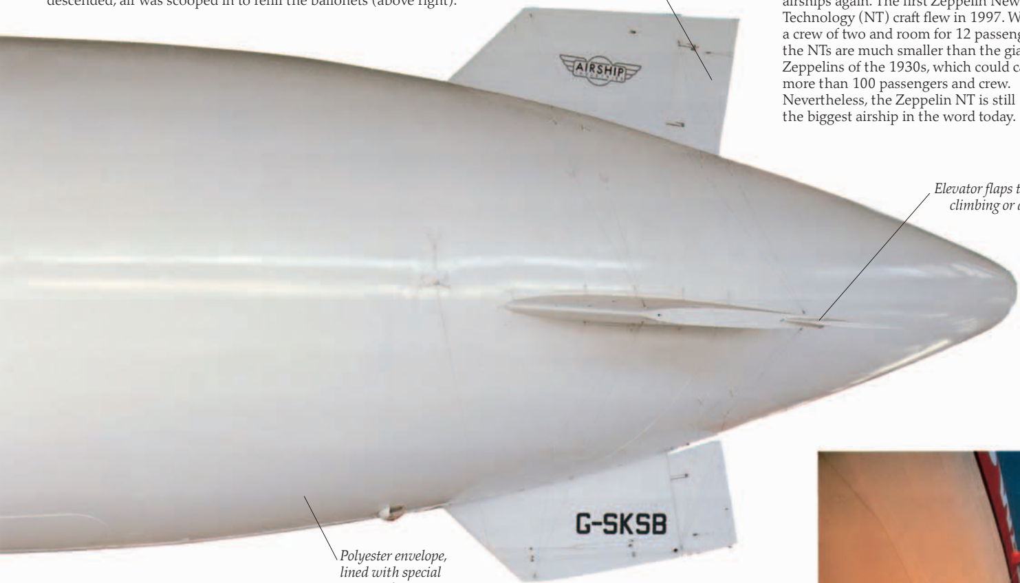
Rudder to steer the airship left or right
