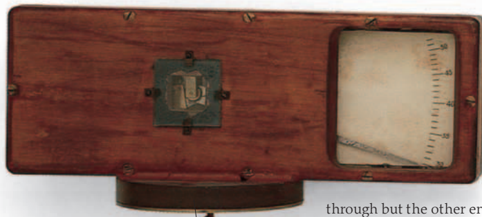
Farnborough airspeed indicator c. 1909
