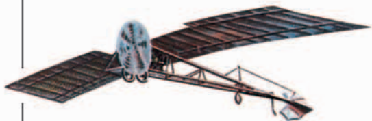
THE FIRST ULTRALIGHT? Brazilian pioneer Alberto Santos-Dumont's tiny No. 19 monoplane had a wingspan of just 18 ft (6 m) and was perhaps the first ultralight. He designed it in Paris in 1907 as an aerial "runaround," and could de-rig it to carry it on his car.
