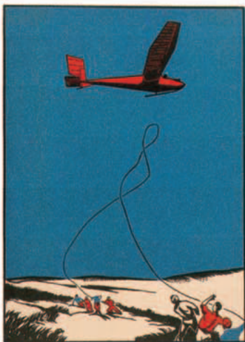
Airbrakes emerge from the wings at right angles, to steepen the descent for landing
