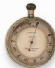
Elliott pocket altimeter c. 1910
