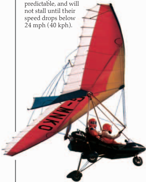
50-hp water-cooled, twin-cylinder Rotax engine Air intake and filter Passenger's seat Pilot's seat Plastic trike cockpit outer shell on aluminum-alloy tube frame Instrument panel Streamlined nose cone Harness Rudder bar
