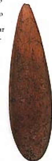
SMOOTHING STONE The rough surfaces left after carving could be smoothed down using a pebble. The highly polished finish of furniture was often achieved in this way.
