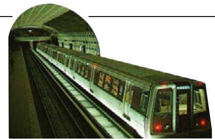
DRIVERLESS TRAINS? Most modern rapid transit systems, such as the Metro in Washington, D.C., are ideal for automation. This is because they have a steady flow of traffic and there is no disruption by slower freight trains or faster express services. The entire network is run by a central computer-based control system, and the trains need no motormen.
