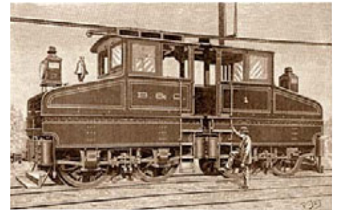
AMERICAN FIRST The first electric locomotives to be used on an American main line were introduced on the Baltimore and Ohio Railroad in 1895 on a section of line 3¼ miles (6 km) long. This short route passed through many tunnels, which had easily filled with fumes when steam locomotives worked the line.
