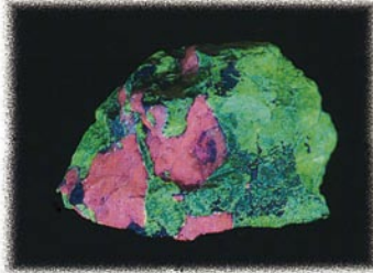
WILLEMITE IN ULTRAVIOLET LIGHT When willemite fluoresces, it emits a bright green light (the pink fluorescence is produced by quartz).
