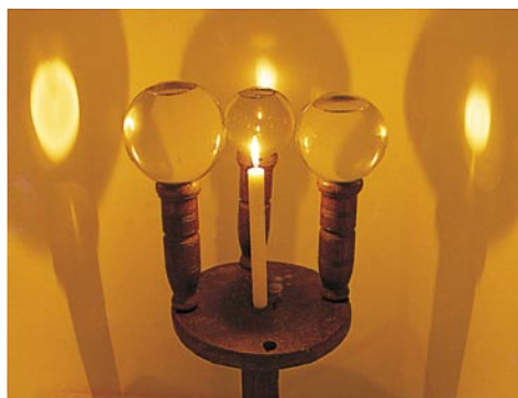
Each condenser focuses light on a different area
