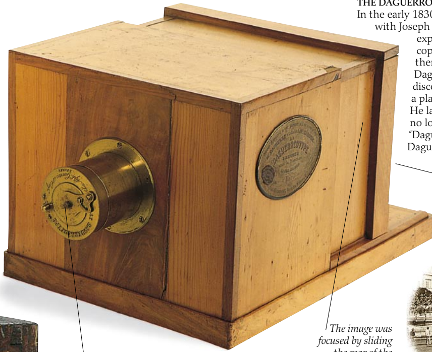
A shutter in front of the lens was moved aside to make the exposure
