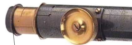
Observer looks at spectrum through tube containing lenses
