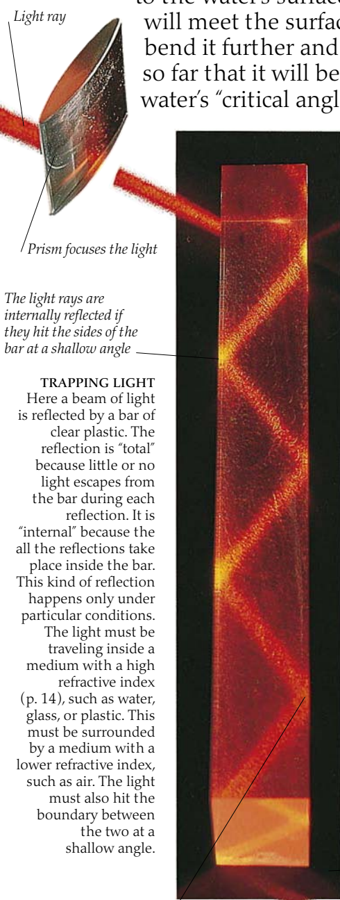
The light rays travel through the end of the bar because they strike it at a steep angle
