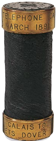
UNDERSEA CABLE Above is a fragment of the undersea telegraph cable that was laid in the English Channel in 1891 to link France and the United Kingdom. Telephone signals traveled along copper wiring housed inside the thick protective covering.
