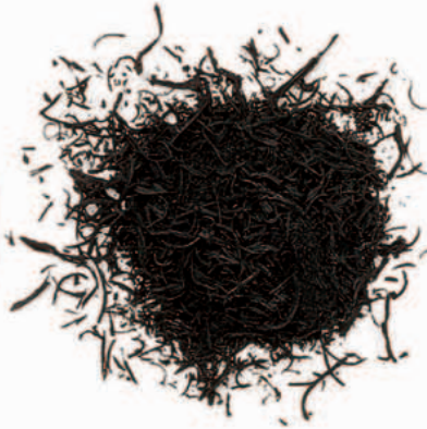
Tire ready to be re-formed after shredding
