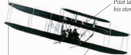
Pilot gently twists wings to control flight
