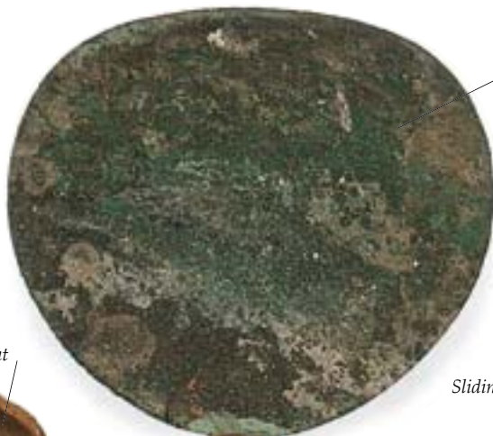
Corroded bronze surface, once polished for reflection
