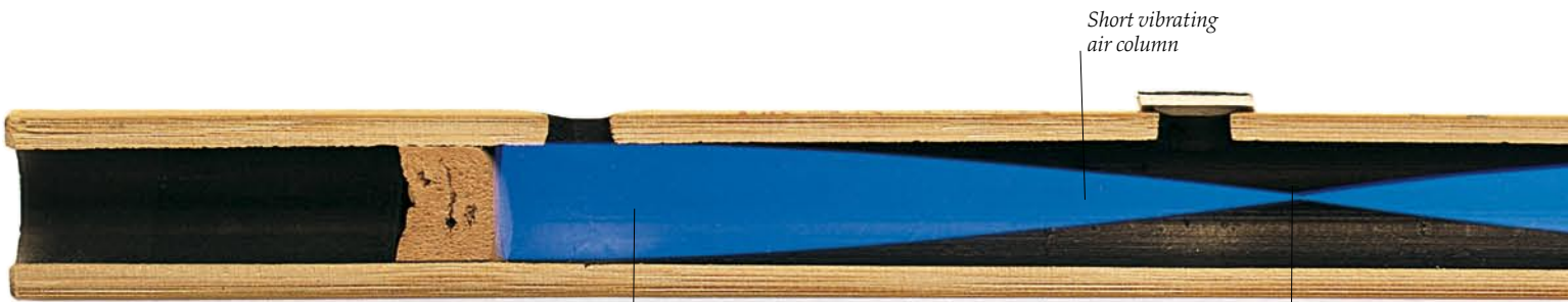
Long pipe sounding over two thirds of length with three holes covered
