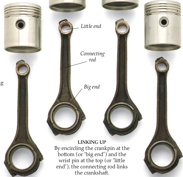
SEALING RINGS To prevent gases leaking out past the piston from the cylinder, each piston has a series of sealing rings.
