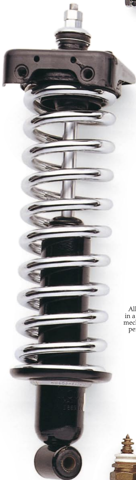
Telescopic shock absorber and coil spring
