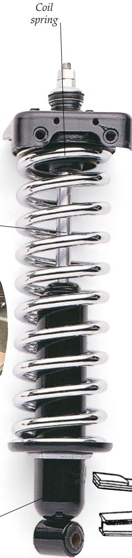
SPRING MATCH above Telescopic hydraulic shocks slot neatly inside coil springs – an arrangement used on most cars nowadays.
