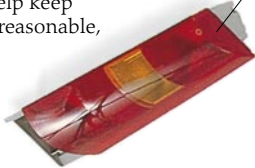
Rear light cluster, including side, turn signal, stop, and white reversing light
