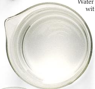
Cerium oxide, very fine polishing powder, used finally to make pebbles smooth and sparkling
