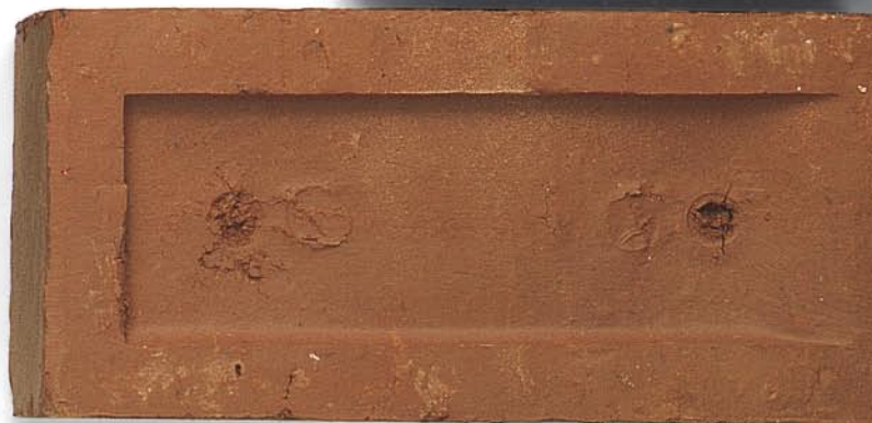
BRICKS Easily moulded clays are fired to make bricks. Impurities in clays produce bricks of different colours and strengths, making them suitable for a variety of uses.
