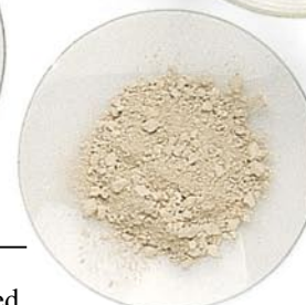
Cerium oxide, very fine polishing powder, used finally to make pebbles smooth and sparkling
