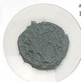
Fine grinding grit used for second tumbling
