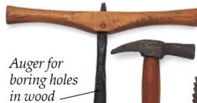
Auger for boring holes in wood
