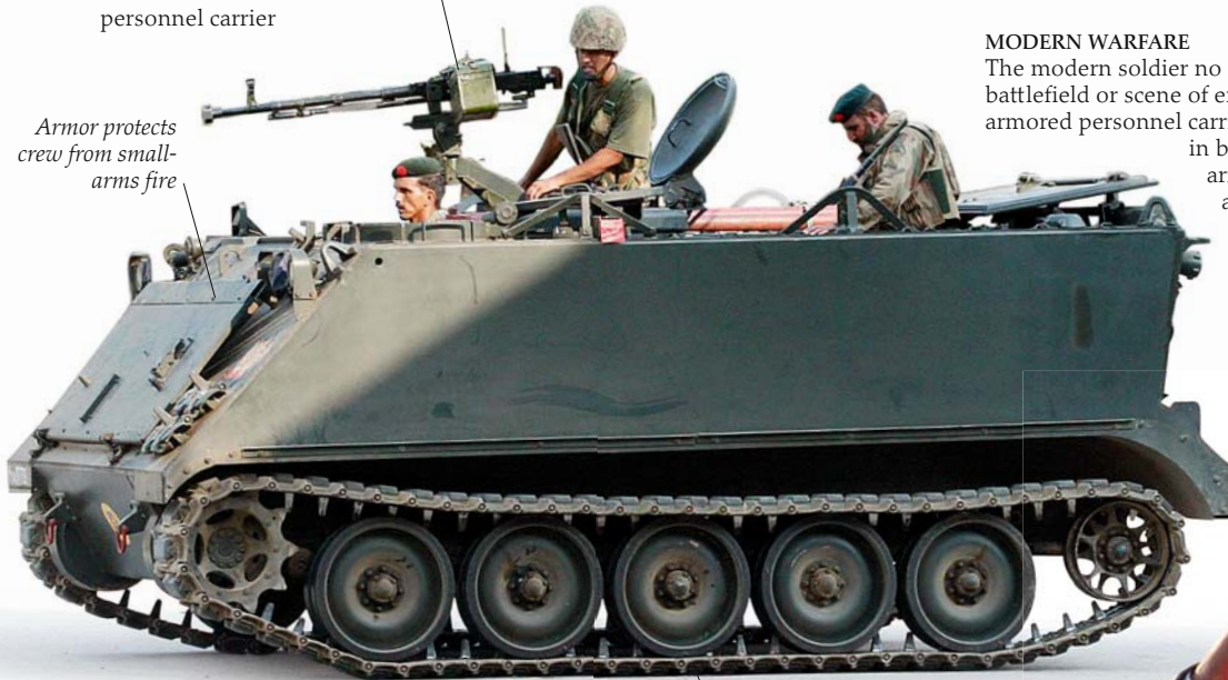
Caterpillar tracks help APC to maneuver on rough ground
