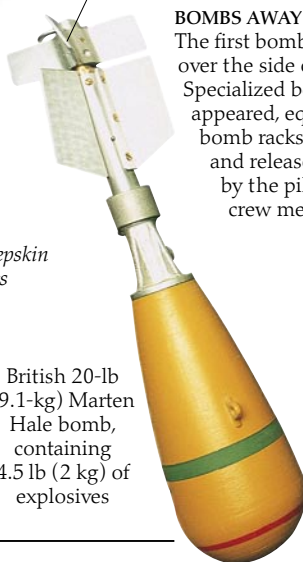
Propeller to guide the bomb
