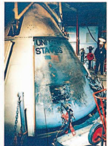
*Effects of the intense heat can be seen on the outside of the command module*
