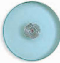
Potential damage of space dust on shuttle window
