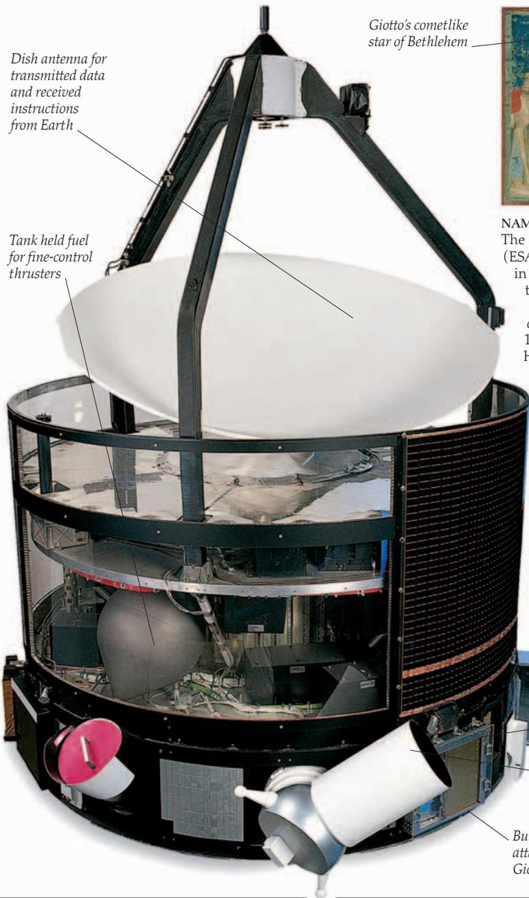
Dish antenna for transmitted data and received instructions from Earth
