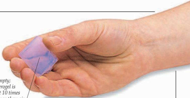
Material used for thermal control on the Infrared Space Observatory (ISO) satellite (p.51)
