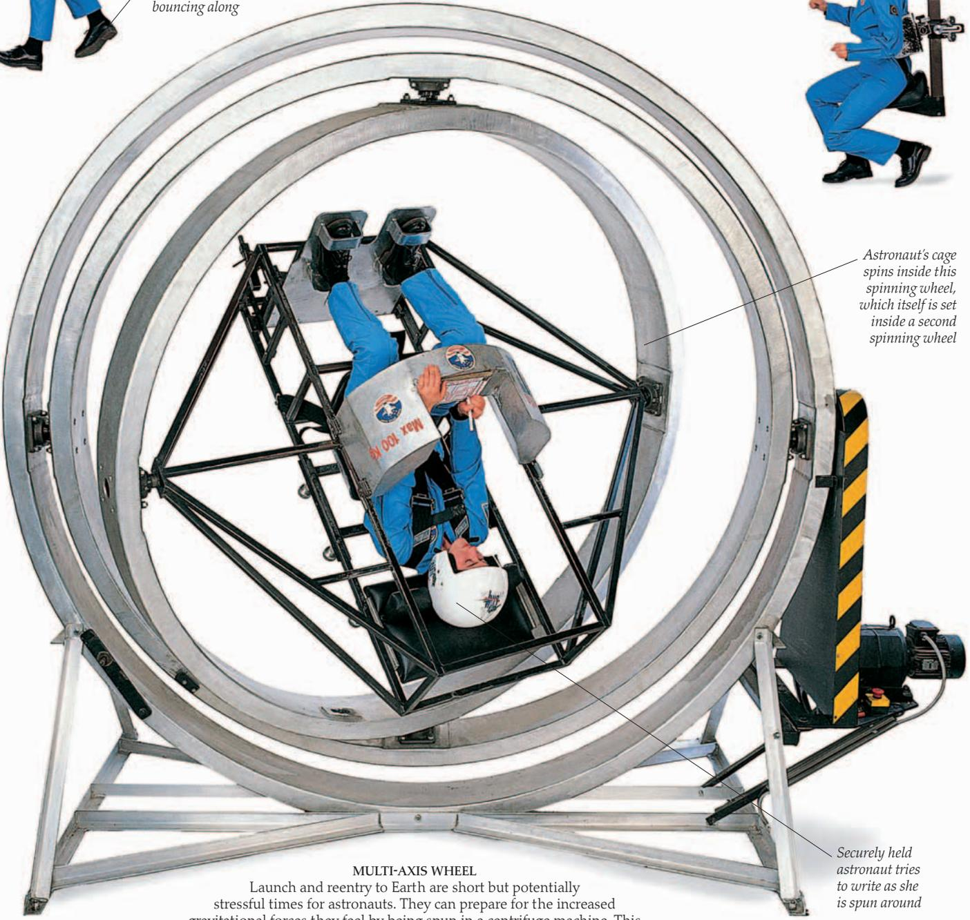
*Astronaut's cage spins inside this spinning wheel, which itself is set inside a second spinning wheel*
