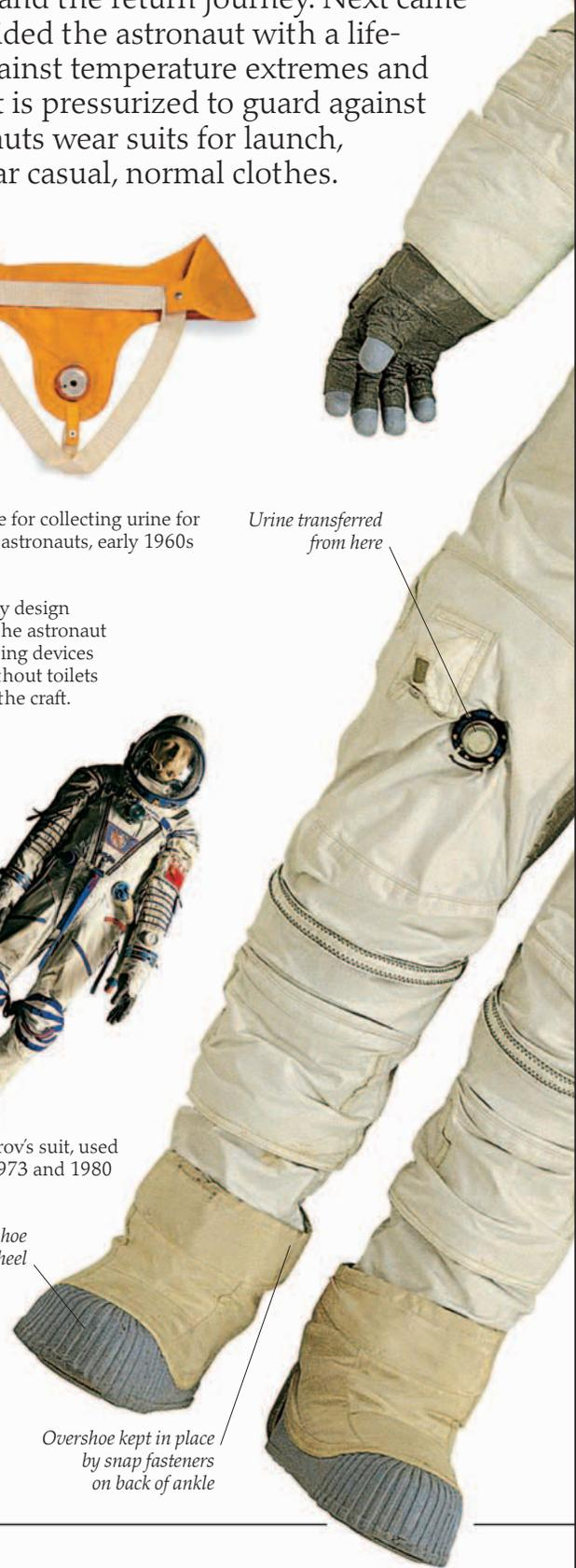
Overshoe kept in place by snap fasteners on back of ankle
