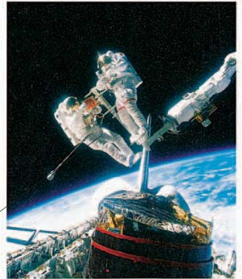
Suits protect astronauts from temperatures ranging from 250°F (121°C) to -150°F (-101°C)
