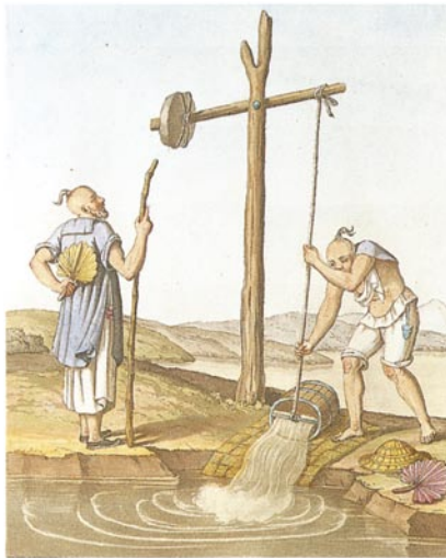
CHINESE SHADOOF People cannot live without a reliable supply of water for themselves, their crops, and their animals (pp. 44-45). Ingenious ways of tapping and distributing water (p. 22) allow life to go on in places that would otherwise be too dry. This simple cranelike device, the shadoof, has been used all over Asia for thousands of years. By adding a weight to the end of a pole, its clever, practical designer made it easy to lift buckets of river water into the irrigation channels that carry water to thirsty crops.
