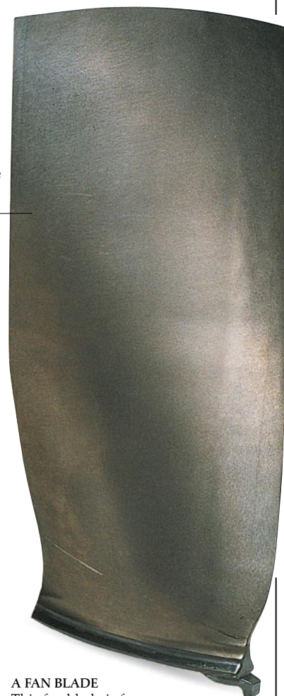
The titanium blade has a hollow "honeycomb" core to make it lighter
