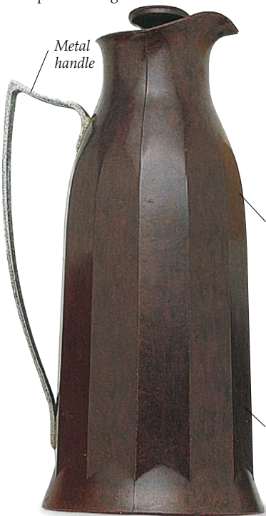
Bakelite can be molded to complex shapes
