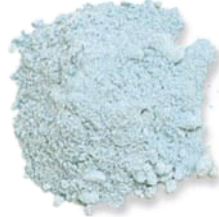
Egyptian blue, containing silicon, copper, and calcium
