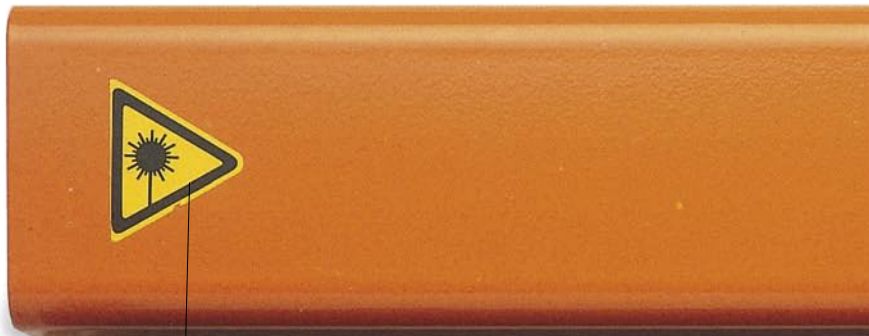
Internationally recognized warning symbol for laser light Laser tube filled with helium and neon Outer tube forms reservoir to replace lost gases
