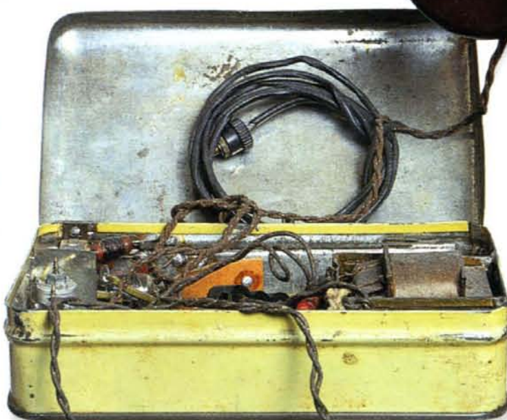
Home-made wireless receiver used by a Dutch family during the occupation
