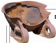
Steel bucket used in gold dredging
