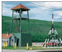
Four-legged “tripod” for determining ice breakup
