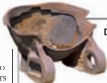
Steel bucket used in gold dredging
