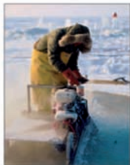
Stress test being conducted on Arctic sea pack ice, Point Barrow
