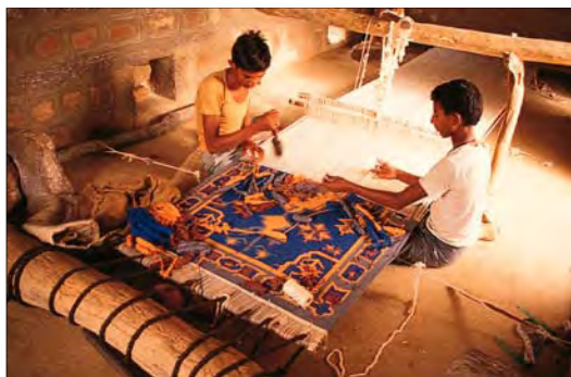
Weaving a carpet on a traditional pit-loom
