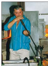
Zwiesel 1 In the old glassworks, which survive to this day, you can watch workers using blow irons to produce vases, jugs and other objects made of glass.
