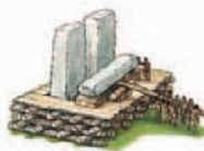
Alternate ends of the lintel were levered up.
