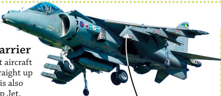
Downward-facing engines help the plane take off.
