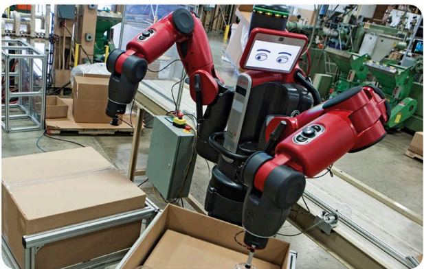
A Baxter robot packs boxes in a factory.
