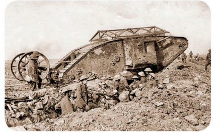
Early 1916 tank with rear steering wheels
