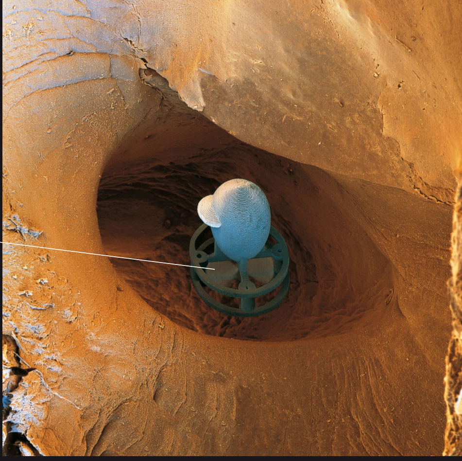
A tiny propeller powers this early version of the microscopic nanorobots that may, one day, explore the circulatory system to find defects.
