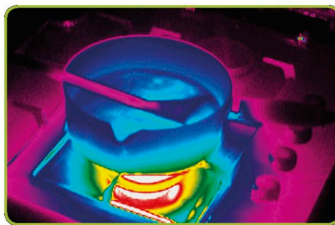
Heat distribution A thermogram (infrared image) reveals how heat is distributed from the hottest point, the flame, to the coldest, the wooden spoon and stove.
