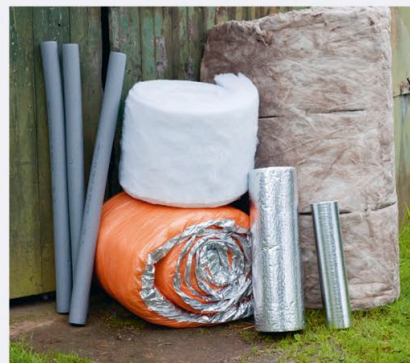
Choose the right insulation: from left, expanded foam for pipework, recycled plastic fleece, a jacket for a hot-water tank, foil reflectors for radiators, and a large roll of sheep's wool loft insulation.
