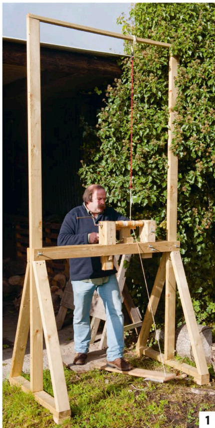
1. A traditional pole lathe doesn't need an electrical power supply and can be set up anywhere, even in the woods. 2. A pine bowl and green wood goblet turned on a pole lathe, with a hand-carved cherrywood spoon. 3. Green woodworking tools , including a froe (top left) for splitting wood and various sharp knives.
