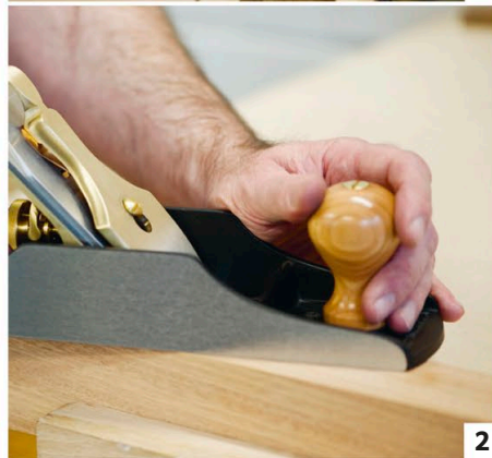
1. Use your thumb knuckle to align a saw as you start to cut. 2. A bench plane smooths rough surfaces. Check your progress by laying the plane on its side to see how flat the wood is. 3. A sharp chisel makes neat work of a tenon (see page 57). 4. Mark wood accurately with a steel rule.
