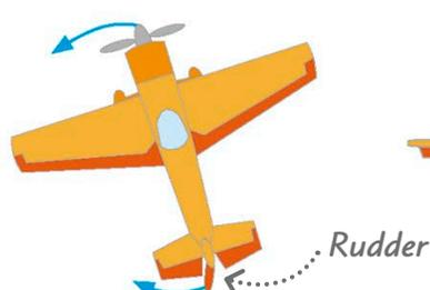
**3** The rudder is an upright flap on the tail. Like a boat's rudder, it steers the plane, making it yaw (turn) left or right.
