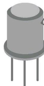
*Large transistors have three metal terminals that look like legs. The transistors in silicon chips are far smaller.*
