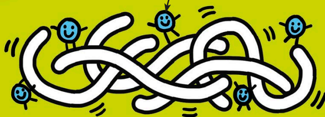
RUBBER POLYMERS SLIPPING AND SLIDING PAST EACH OTHER
