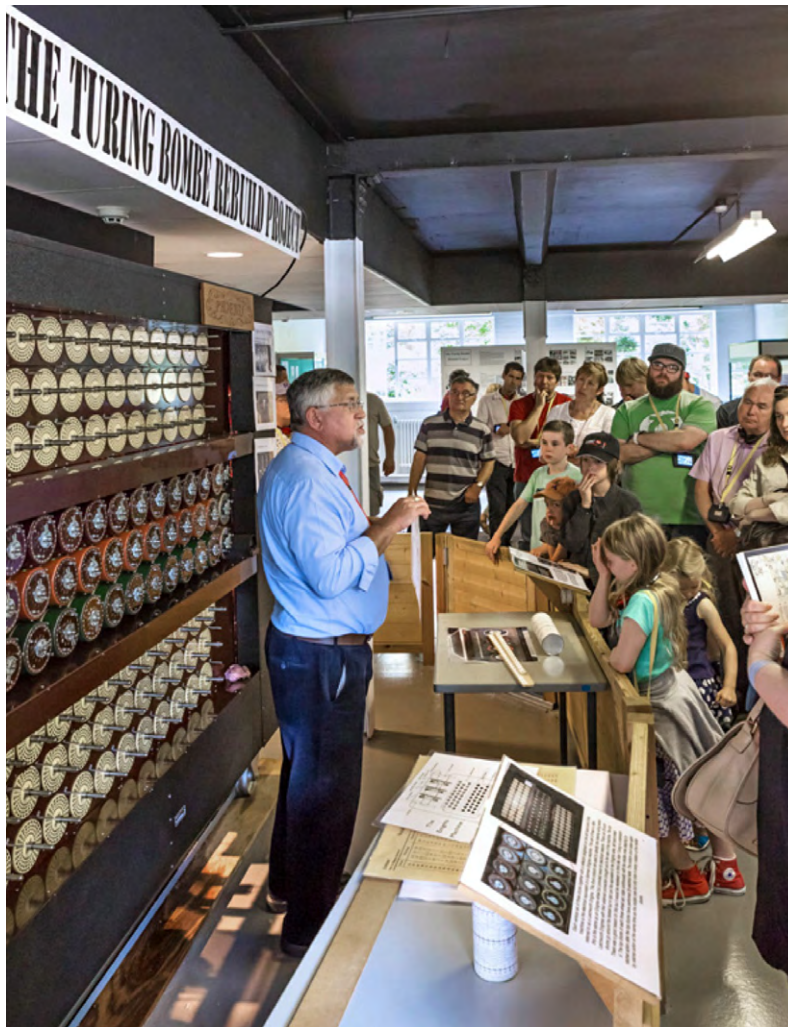
A Turing Bombe , used to decipher coded messages, has been rebuilt at the museum at Bletchley Park, the British code-breaking center during World War II.
