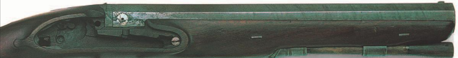
LOCK left Screwed to the side of the stock was the lock—the mechanism that fired the pistol. When the trigger of a flintlock was pulled, the cock swung forward, making sparks by scraping the flint down the frizzen, or steel, and pushing open the pan cover. The sparks fell into the priming powder, which burned with a flash and set off the main powder charge in the barrel, through the small "touch-hole."
