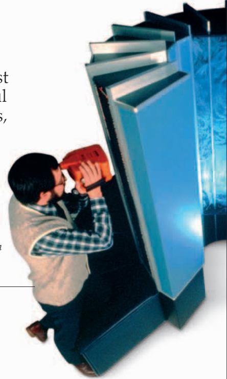
Engineer uses an infrared viewer to search for overheating in a Cray supercomputer
