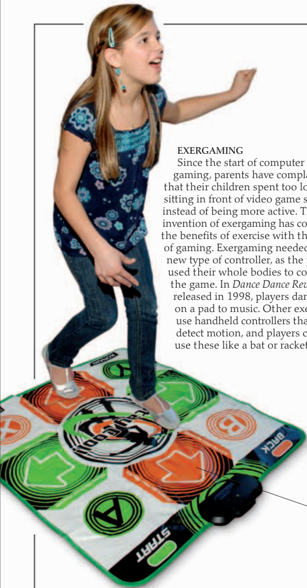
Each area of dance pad, or stage, is sensitive to pressure
