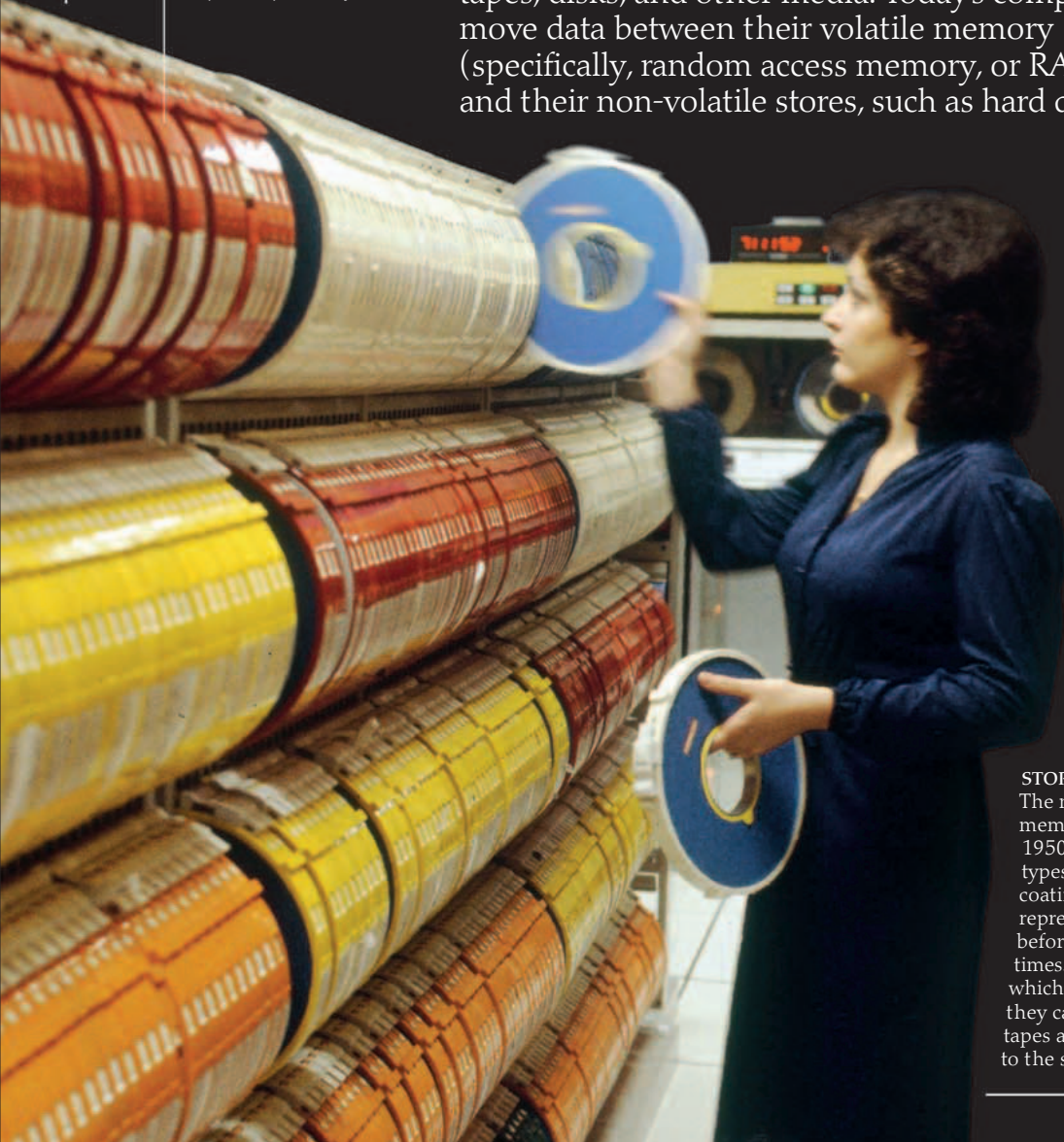
Magnetic data storage tapes in a rack, in a computer tape library
