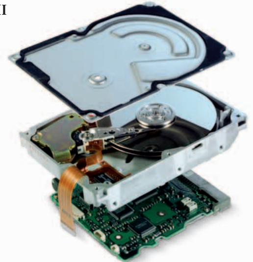
Layered view of hard disk drive
