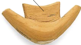
Wooden mouthpiece to hold drill in place
