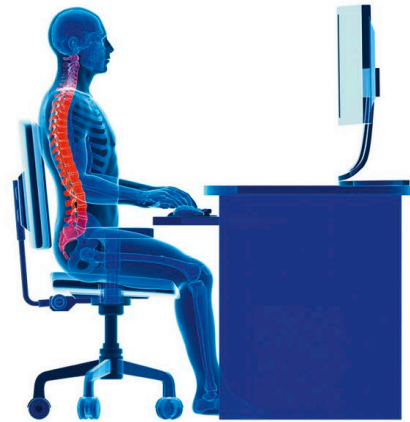
ERGONOMIC SEATING takes into account the sitter’s elbow height, seat height, thigh clearance, eye level, and back support.
